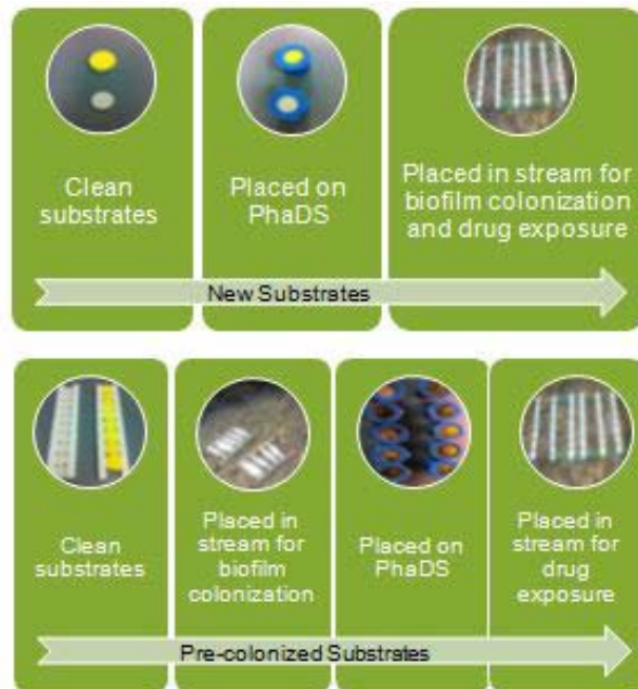
FIGURE 1. An overview of the methods for preparing new substrates and pre-colonized substrates.
