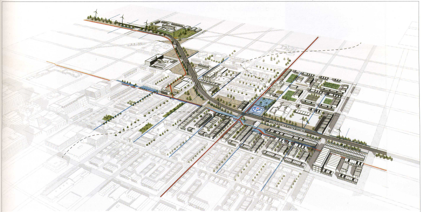
FIG. 12. A design combining: rooftop- and soil-based water harvesting, filtering, and storage; greening and recreational space; and wind energy capture. Plots for biofuel and urban agriculture are also provided (Design: Sven Augusteyns, Parsons—KU Leuven design project, supervised by B. McGrath).
